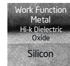
XTEM of I/O dielectric stack
